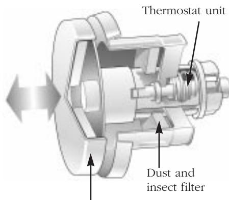
The valve head is insulated against condensation and noise
